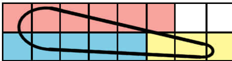
Figure 4: The top of the wing is painted red, the bottom blue. The nodes colored yellow contain two surfaces, so the paint there will depend on the order of application.
