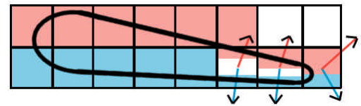
Figure 5: Nodes with two surfaces contain two color samples, with an associated normal.
